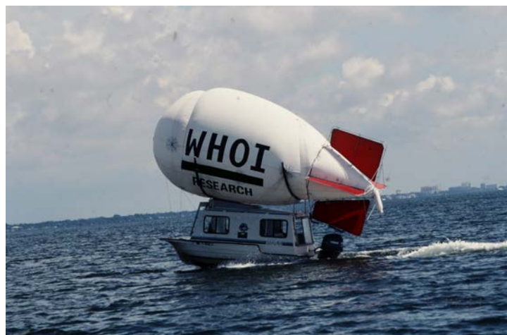
Above "The Blimp" in transit, cradled on our aircraft carrier, R/V Hobo. To the left shows "The Blimp" deployed.
