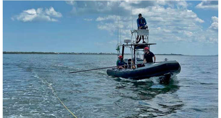
Jonathan Crossman with a specialized cutting tool attached to a pole at the bow of the boat practicing whale entanglement cuts on a towed line.
