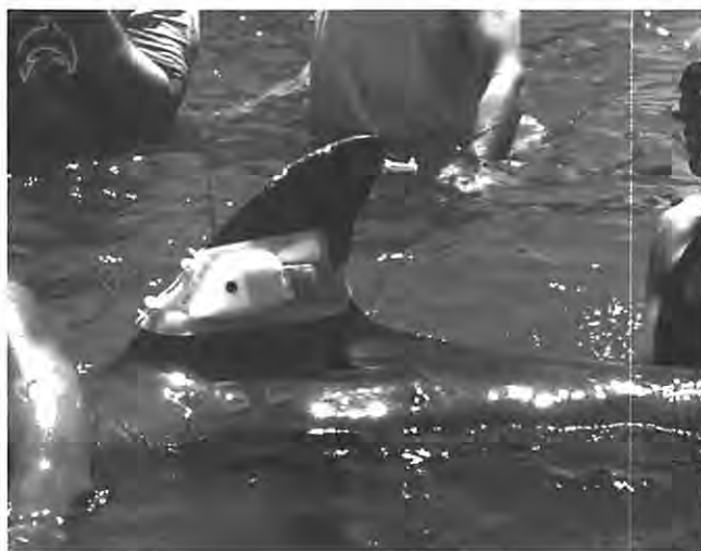
Figure 1. A thermal logger positioned on the dorsal fin of a male bottlenose dolphin.
