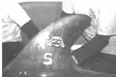
Figure 2. Satellite-linked transmitter on "Betty's" dorsal fin.
