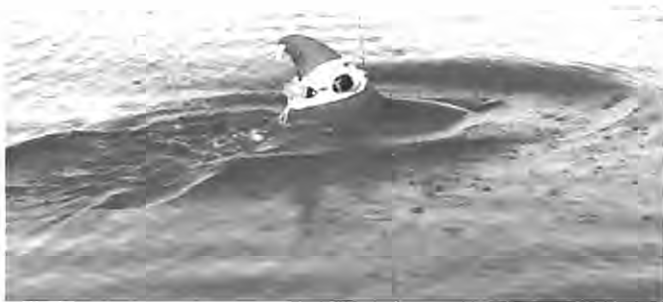
The suction-cup-mounted Trac Pac records data on dolphin behavior and stomach temperatures.
