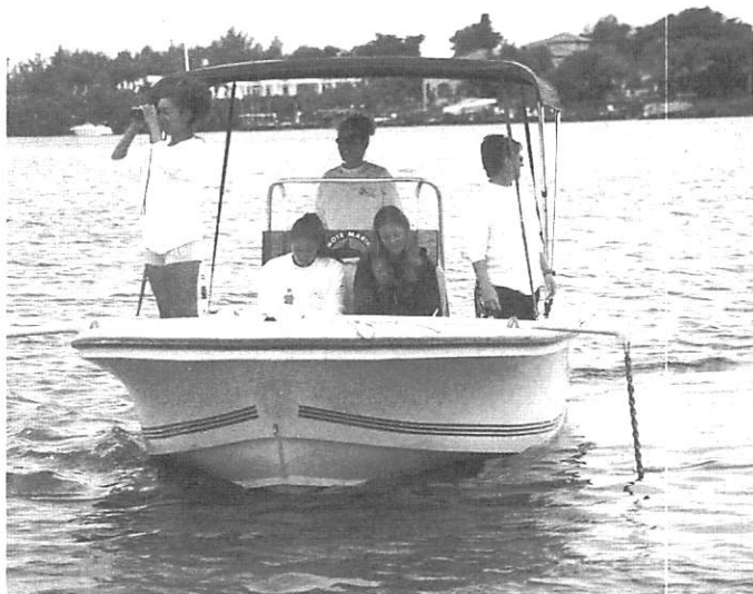
Research team studying the acoustic communication of wild dolphins. A hydrophone was towed on each side of the boat, separated by a 3-m PVC pipe tied across the gunwales at the bow of the boat
