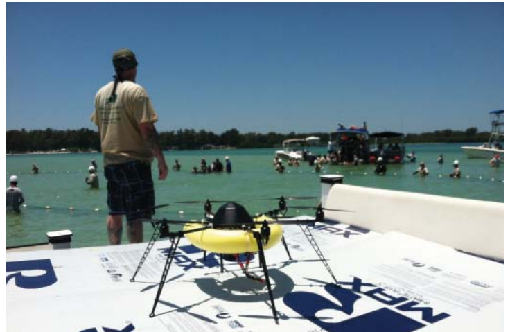
Unmanned aerial vehicle imaging system, a six-rotor remote-controlled helicopter with a downward-facing digital camera, developed by researchers at the Duke Marine Lab and the Woods Hole Oceanographic Institution to measure dolphin body condition.
