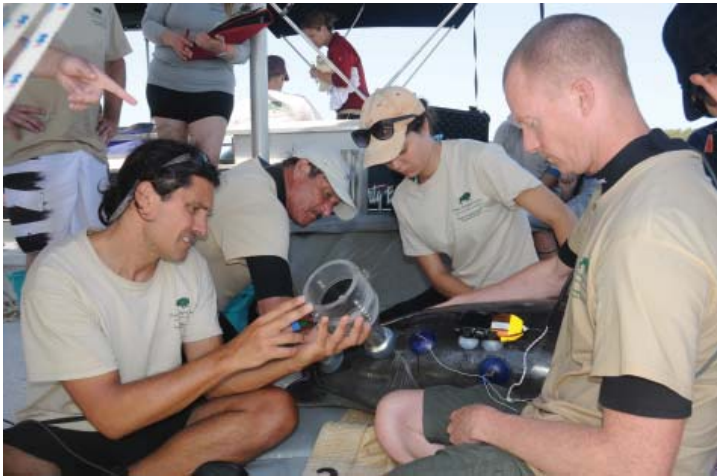
Dr. Andreas Fahlman collecting respiration data from F185 using a pneumotachometer.
