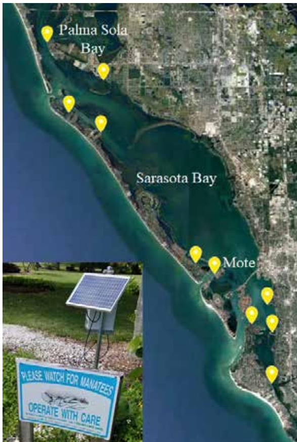
Each yellow marker represents the location of an acoustic monitoring station. In the bottom left corner is a picture of one of the newest stations. The solar panel powers the station, the grey box houses the battery, memory cards, cell modem, and processor, and the manatee sign shows this resident's commitment to manatee conservation.
