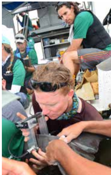
James Powell tests his bone sonometer on a dolphin's peduncle while colleague Spencer Fire collects the data on his computer.
