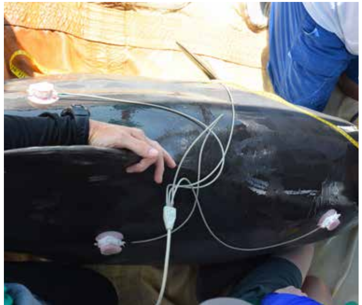
Suction cup sensory electrodes positioned on a dolphin's back for ECG monitoring and recording.
