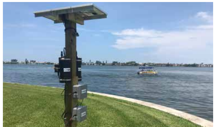
Top: Single camera view from a small-scale electronic monitoring system deployed by FlyWire Cameras on R/V Flip during fish monitoring surveys in Sarasota Bay. Bottom: Shore-based electronic video monitoring system.
