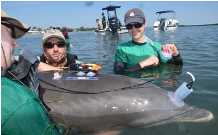
F164 freshly fitted with a Dtag by Julie van der Hoop prior to his release. The Dtag is recording the breath sounds at F164’s blowhole to monitor his respiratory function. The suction cup on his melon is a hydrophone that records his vocalizations for communication studies.
