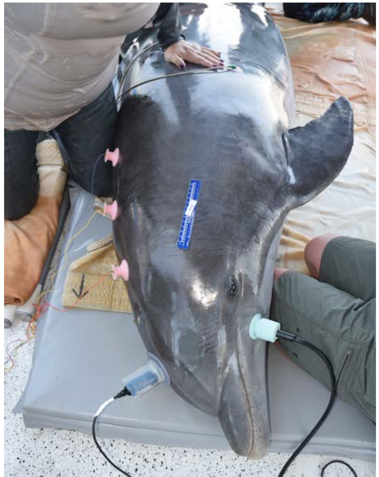
F173, showing placement of the jawphone on the lower left jaw and AEP sensors on the animal's dorsal surface. A recording hydrophone is located on the melon of the animal, and ECG sensors are located behind the pectoral fin.
