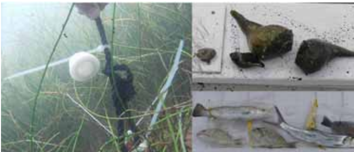
Left: the white circular DGT probe is about one inch in diameter. Top right: benthic organism samples. Bottom right: fish samples.
