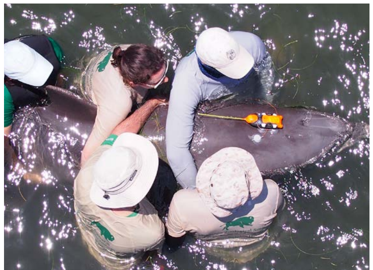
F254 wearing an EKG DTAG3, just prior to release. Unlike traditional DTAGs, this modified tag includes two peripheral suction cup electrodes for measuring heart rate, one of which can be seen here to the right of the main device.
