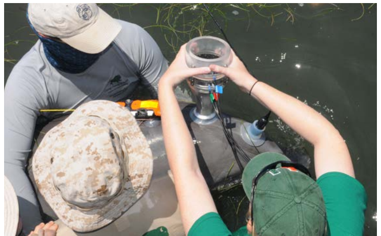
A device is placed over this dolphin's blow hole in order to measure oxygen concentrations as the dolphin inhales and exhales. These data can then be used to determine the animal's metabolic rate.
